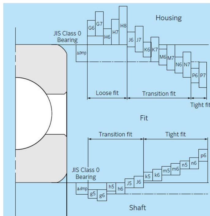
Parameters you often see on a bearing or bearing spare part drawings:
