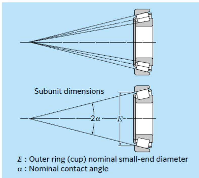
How to understand the code of metric size taper roller bearing:
