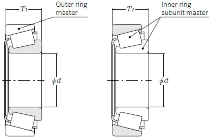
Table 6.6 Tolerance of tapered roller bearings (inch series)
